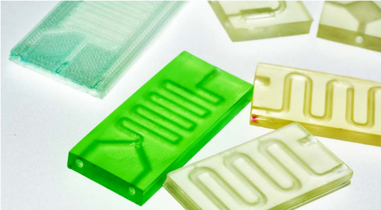
Lab-on-a-chip microfluidic devices are designed to be more representative of the biochemical environment found in living tissues.
