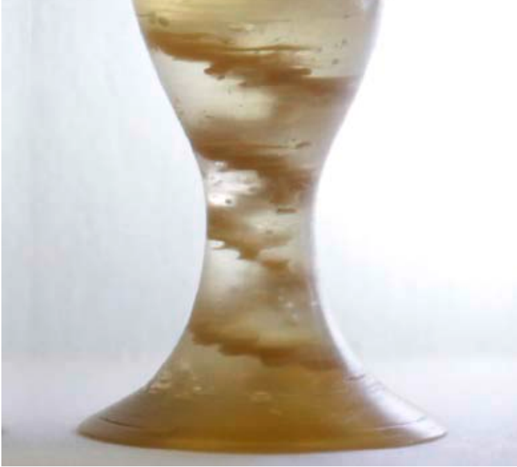
MM-3D printed object with internal helicoidal staircase (A. Studart/ETHZ).
